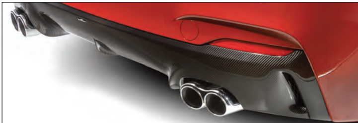
Carbon rear diffuser, silencer with 2 "Racing Evo" tailtrims
