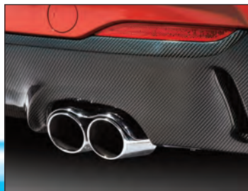
Carbon rear diffuser, silencer with two "Racing Evo" tailtrims
