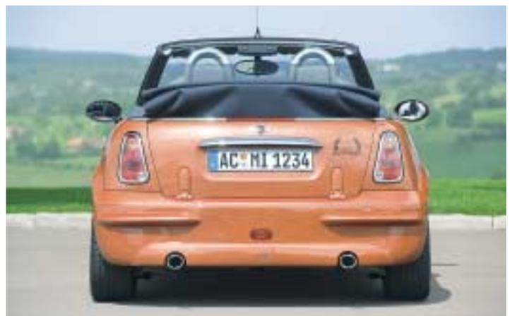
*Striking front, dynamic rear: With aerodynamic components of PU-rim and twin pipe exhaust system of V2A with chromed tailpipes.*
