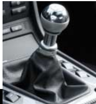
Aluminium gear knob and carbon fibre trim for the dashboard, centre console and side panels.
