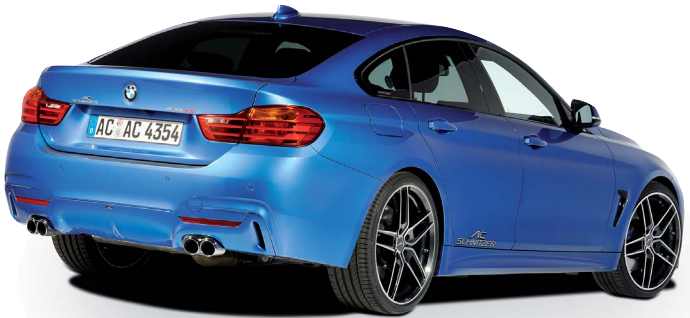
Rear skirt protection foil, rear diffuser (M-Technik), silencer with two "Racing Evo" tailtrims
