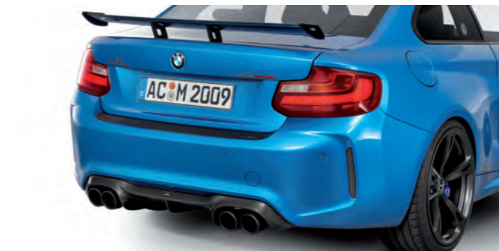
Carbon rear wing (export), rear skirt protection foil, carbon diffuser, "Sport Black" tailtrims
