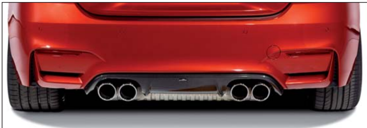
Carbon rear diffuser, twin silencer with 2 "Sport" tailtrims each, in right/left combination
