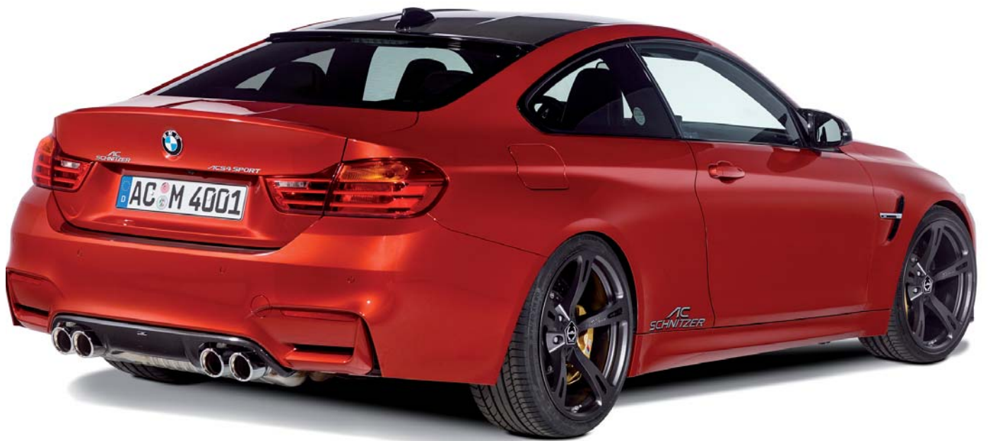
Rear roof spoiler, rear skirt protection foil, carbon rear diffuser, twin silencer with 2 "Sport" tailtrims each, in right/left combination
