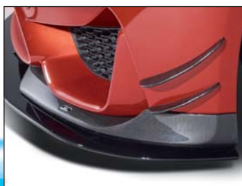
Carbon front spoiler, front splitter (racing version), carbon front side wings 2 pieces each side (racing version)
