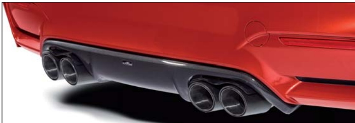
Carbon rear diffuser, twin silencer with 2 "Racing Evo Carbon" tailtrims, in right/left combination
