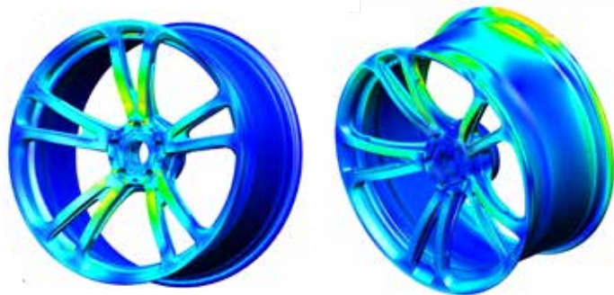
FEM analysis AC3 “Evo” Lightweight Forged Wheels
